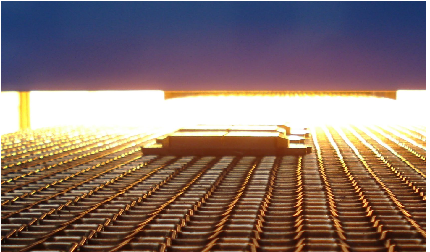
Cosworth brake pads undergoing the heat searing process
