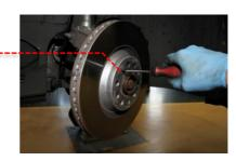
4 Remove the three T30 torx bolts holding the backing plate in place
