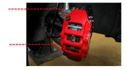
9 Remove the OE brake line from the car using 11mm spanner and install the new Revo brake line. If any brake fluid if spilt be sure to clean up immediately as can be corrosive.
